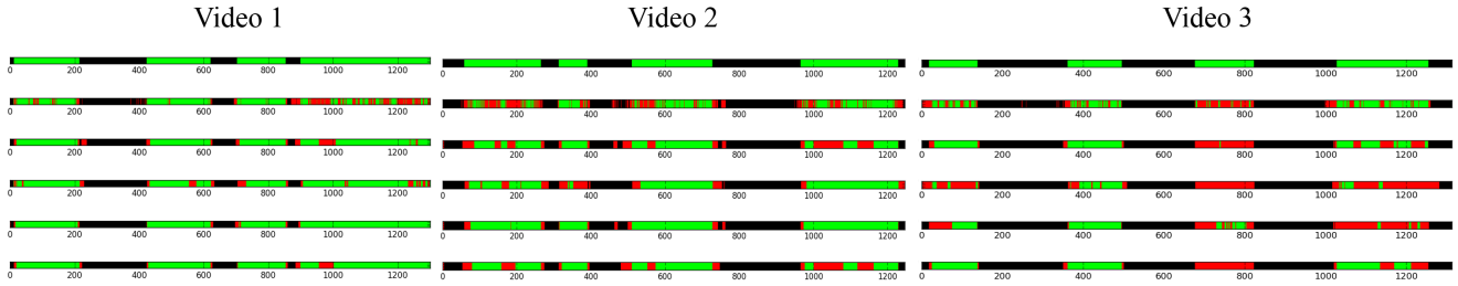
Figure 7. Comparing different sequence labeling results. Black is background, Green is an action, and Red is false prediction. First row: ground truth. Second row: labeling results with CNN only. Third row: labeling results with added LSTM. Fourth row: attention LSTM labeling results. Fifth row: instance-aware labeling results. Sixth row: Smoothing applied on basic LSTM results. Video 1 and Video 2 illustrate how joint prediction can help improve accuracy by considering global information at instance level. Video 3 shows a failure case due to poor-quality detections.
